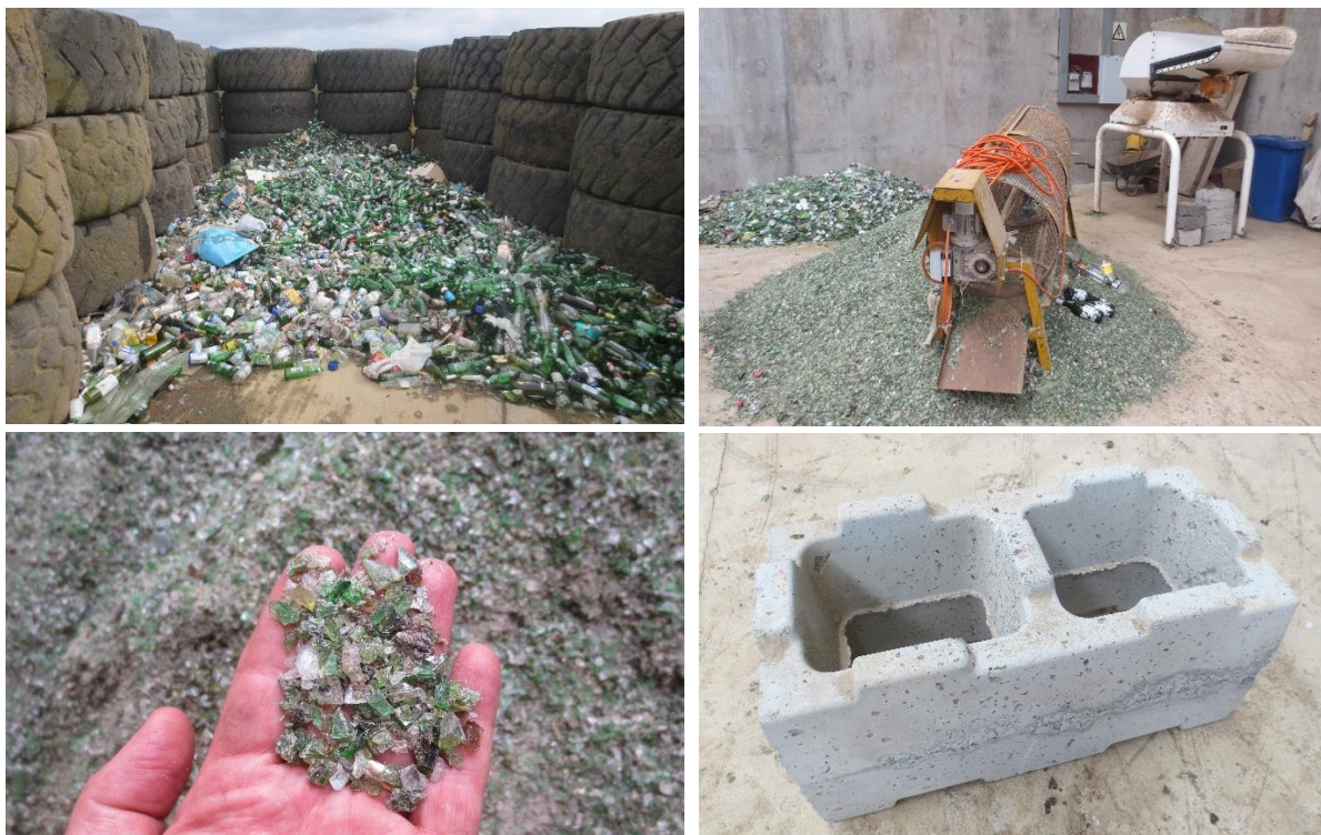
Figures 26-29: St Helena glass storage and recycling. Fig. 26 (top left): Collection bay at Horse Point waste site. Fig. 27 (top right): Inside the large shed at Horse Point – glass imploder (crusher) at the back right of photo, with a rotating screen and pile of screened crushed glass in foreground. Fig. 28 (below left): Crushed and screened glass. Fig. 29 (below right): Concrete block made using recycled and crushed glass as 25% of the aggregate.
