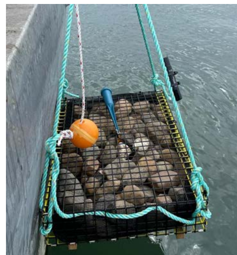
Figure 16 – European Lobster Settlement Index (ELSI) project sampling equipment. Left: settlement collector (wire mesh filled with cobbles of various sizes). Right: Neuston Plankton Tow (conducted at dusk).
